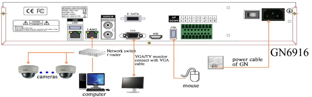
**Step 1:** Follow above to install cameras to the video ports of TeleEye GN.
