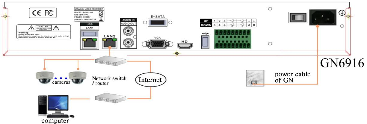
**Step 1:** Configure the network settings of TeleEye GN through PC with LAN connection.
